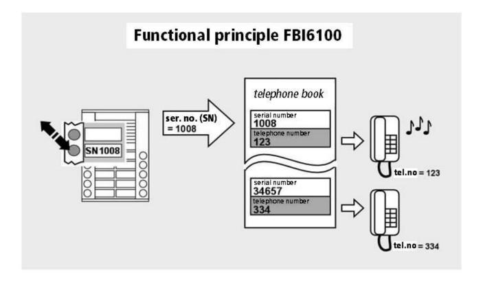
By using the programmed call buttons of the connected door station, a call to an allocated remote station can be triggered. For this, the SIP-Gateway manages a corresponding list of telephone numbers (telephone book) which are assigned to TCS:BUS serial numbers. From the remote station, the communication can be terminated early via DTMF-commands during a conversation. It is also possible to trigger the door opener or operate the light switch relay.
