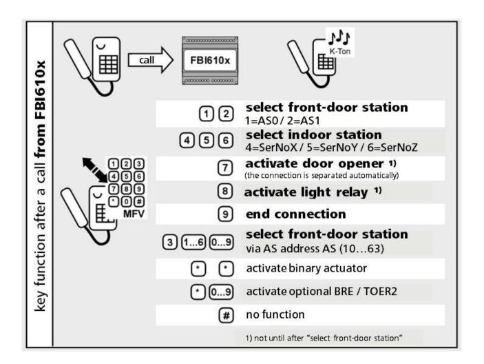
For using the binary output a configuration is necessary, see *settings hardware*, *system*.
