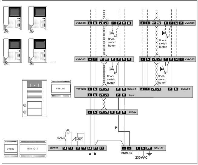
Wiring diagramm 5-wire-connection
