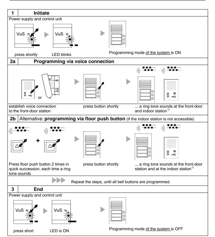
1) If a Progsperr tone sounds instead, a programming lock is set in the front-door station. The programming lock can only be removed with the Service Device TCSK-01
