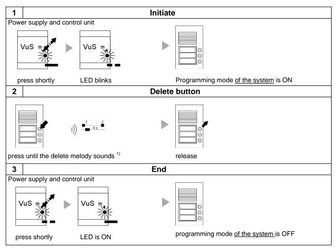
1) If a Progsperr tone sounds instead, a programming lock is set in the front-door station. The programming lock can only be removed with the Service Device TCSK-01 or the configuration software configo™.
