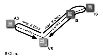
max. 65 m distance AS-VS on 0.6 mm diameter max. 115 m distance AS-VS on 0.8 mm diameter
