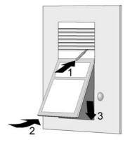
Never seal the device using silicon! Condensate must be allowed to drain and evaporate.
